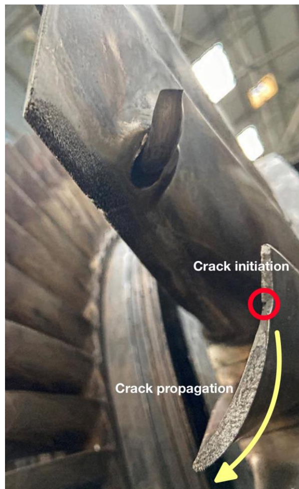
Fig. 1. In the photograph, a fracture is visible about 100 mm from the root of the turbine blade on the exhaust side of the steam turbine.
