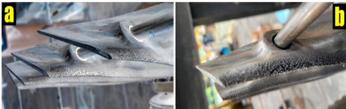
Fig. 1. In the photograph, a fracture is visible about 100 mm from the root of the turbine blade on the exhaust side of the stream turbine.
