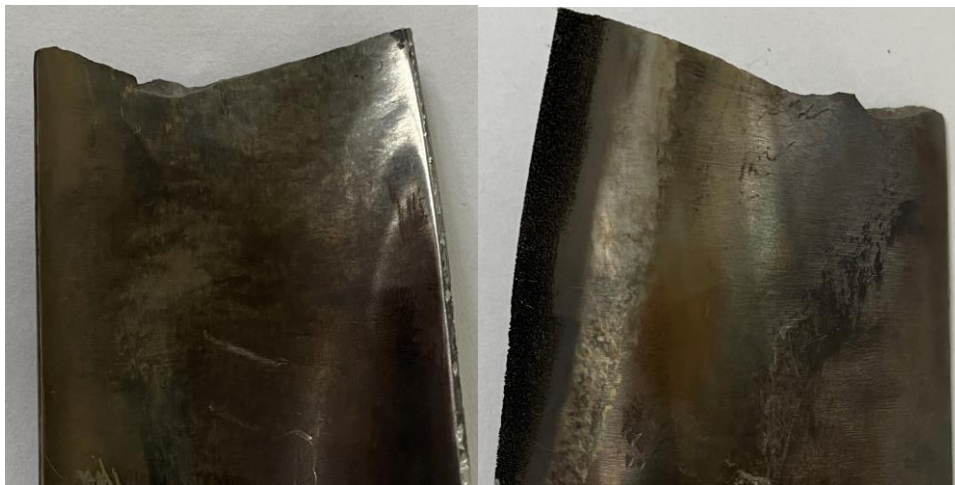
Fig. 2(a, b, c). The leading edges of turbine blades located on the exhaust side show several pits/grooves, an apparent fin-like texture.
