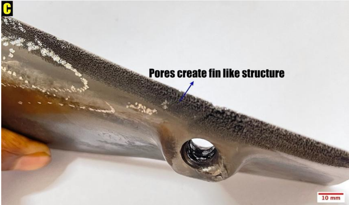
Fig. 2(a, b, c). The leading edges of turbine blades located on the exhaust side show several pits/grooves, an apparent fin-like texture.
